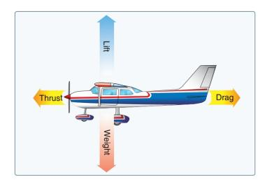
There are four forces that act on an aircraft when it is in flight. These forces are lift, weight, thrust and drag. During straight and level flight the four forces of flight are in balance. When these forces become out of balance the aircraft will leave level flight and the following situations may occur:
